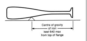
E.3.4.2 For boats first measured after 1st March 1994 the keel casting shall be weighed, measured and numbered before being fixed to the boat. The number shall be engraved on the port side at the location of the upper template, 200mm from the aft edge of the keel.
